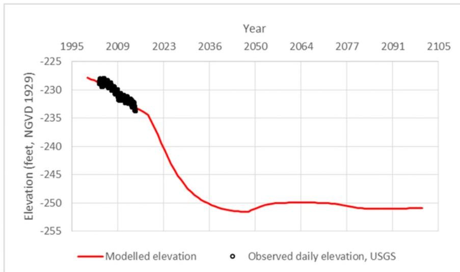
Figure 4: Elevation change over time predicted by the SSAM utilizing implementation: baseline flow scenario.
