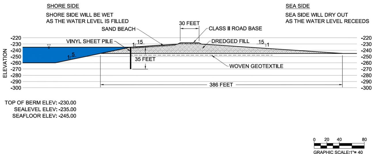
Figure 15: Levee Cross-Section Configuration with Seepage Barrier
