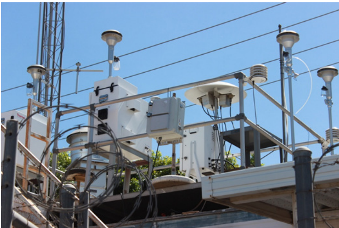
An IVAN AIR community air monitor was colocated with a regulatory air monitor from the California Air Resources Board (CARB). The community air monitor is the smaller gray box attached to the front railing (center of photo). The surrounding equipment is part of the CARB regulatory monitor. Colocation is important for data quality assurance. Photo courtesy of Comite Civico del Valle.
