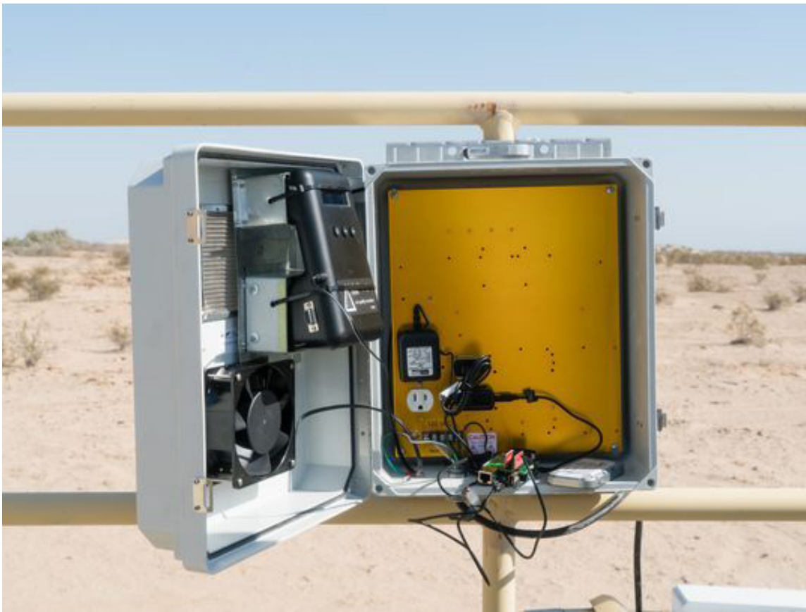
A community air monitor assembled in Imperial County. The Dylos sensor and fan are located on the left side of the opened enclosure and connect to the power source on the right side. The enclosure protects the monitor in the harsh desert environment. Photo courtesy of Zoe Meyers/The Desert Sun.
